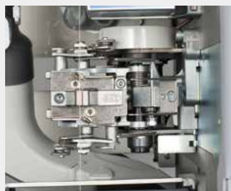
The Mach Splicer uses compressed air to loosen the ends of spun yarn to a fibrous state. Then, by joining together the loosened ends and blasting them with compressed air, the fibers are integrated (twisted) and many types of spun yarn can be joined together without knots.
