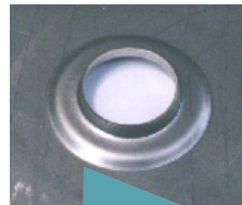
[EX.5] \Phi 19.5 & \Phi 36 h3.0 (1) Pierce → (2) Burring & Emboss
