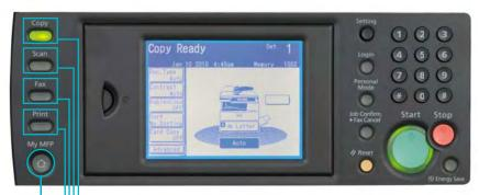
The MFX-2570 and MFX-2550 have a 5.8" backlit touch screen display which guides the user quickly and easily through the machine settings, job processes and error management. By pushing the backlit buttons you can simply change between the modes, see the job status and change settings.
